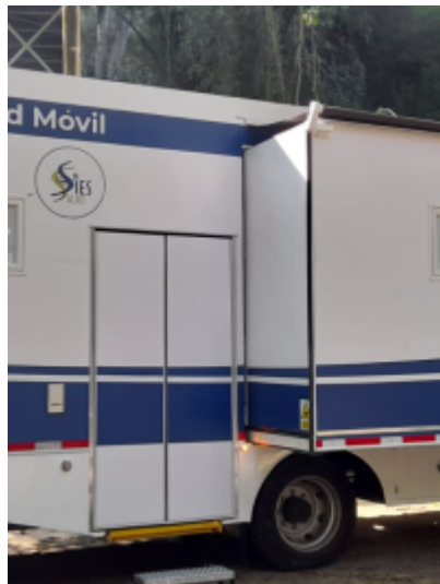
Rear-lateral view of the unit with the expansion module fully deployed, revealing the scale of operational space available in the field.
