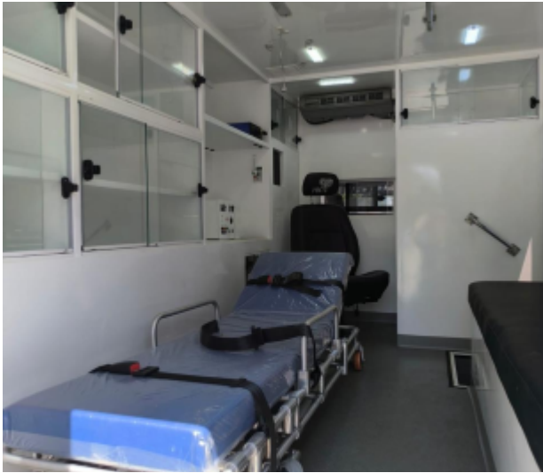
Medical module interior: glass cabinets for ECMO supplies and certified stretcher
